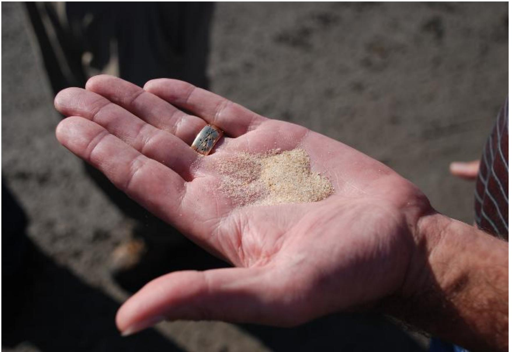
Oil and gas “proppants” are used to hold open the tiny fractures created during a fracking operation.
